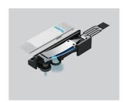
The rotary drives in the cobot are controlled with piezo valves. Piezo valves have several advantages over conventional solenoid valves: they're small and lightweight, highly durable, incredibly fast, energy-saving and highly precise. This "controlled pneumatics" technology permits precise positioning of the rotary drives.
