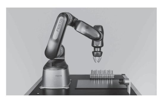
In this exhibit, the Festo Cobot recognises and sorts different fruits based on their outline. The third-party camera system used can be easily put into operation with the help of plug-ins without much prior knowledge.
